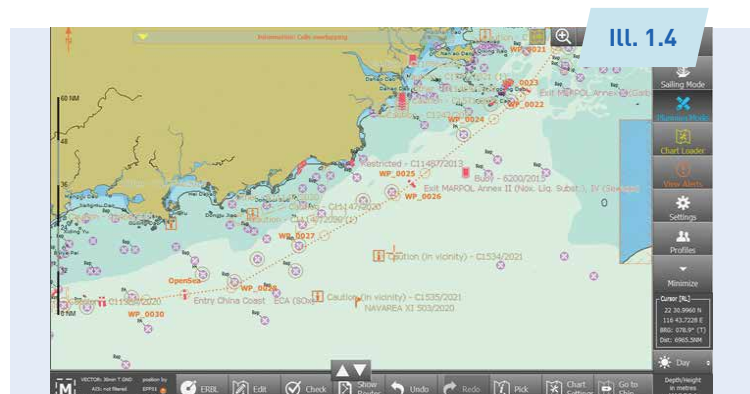
Plotting T&P NtM and NAVAREA as an ECDIS overlay
