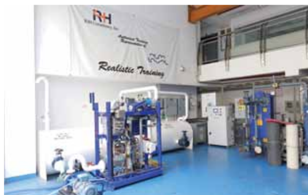
New ballast water system simulator at UMTC
